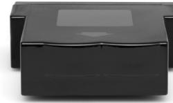
**1** Determine the best location for the Radar Receiver. The best location is typically under the bumper or inside the front grille of the vehicle. For the best radar performance install the Radar Receiver with the label facing up and the arrow pointing forward, and provide a clear "view" of the road (see photo at right).
